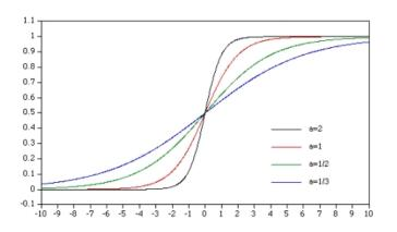
Notice that different choices for the input to the sigmoid (labeled a in the diagram) result in different shapes of the sigmoid. Why is this good for prediction? Different choices  $\beta$  give sigmoids of different "steepness"; logistic regression finds the steepest curve that fits the data
